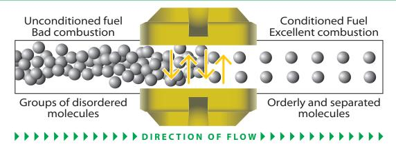
These two beneficial effects of the intense magnetic field mean that many more of the fuel molecules entering the boiler will readily react (i.e. combust) with oxygen molecules. This leads to more heat being released in the boiler and consequently a hotter flame. (This rise in temperature is well within the boiler's operating tolerances).
